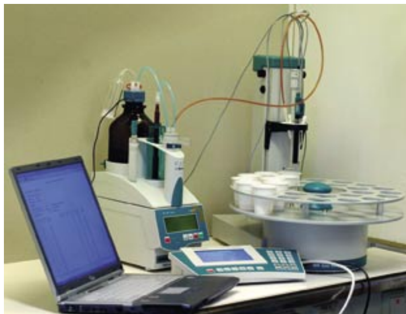
The Sintalyzer system for fully automatic fluoride determination.
